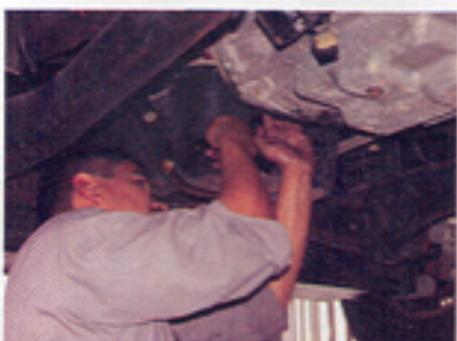
5 Rotating the transmission end-shaft allows access to each of the torque converter's bolts to free the transmission from the engine.
