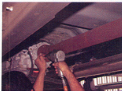
1 Our first step to installing the Precision torque converter was to take our truck to Inglewood Transmission Service where they began by unbolting the driveshaft from the transmission.
