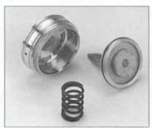
While not trick, the "A" servo from the Thunderbird Super Coupe AOD is a standard upgrade item everyone, including Precision Industries, uses to apply more clamping force on the overdrive band.
