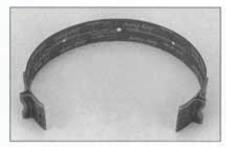
With more clamping force comes a need for increased holding force. This is supplied by a 1 3/4-inch, Kevlar-lined overdrive band in place of the stocker.
