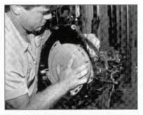
Dennis fitted the Stallion converter onto the input shaft and front pump hub, watching for complete engagement before attempting to install the fresh AOD into our LX.
