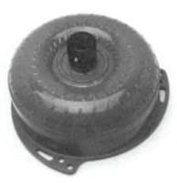
doing the same at 2000 RPM. That is why a stock size higher stall lock-up must be engineered to be much stronger and contain more bullet proof parts than the stock converter. It has a much tougher job to do and live!
