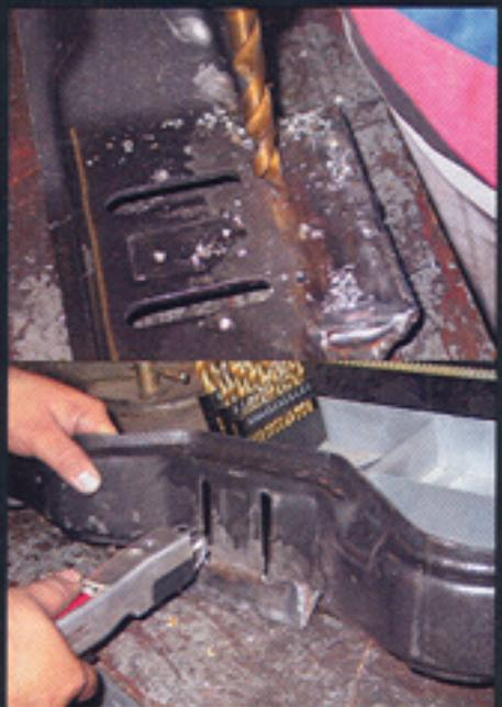
▲ Saul bores holes through the newly fabricated extension plate, then uses an air saw to elongate the slots for the transmission mount.
