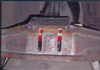
▲ Now that the tranny mount is properly aligned, it can be secured to the crossmember—and we can go home!
