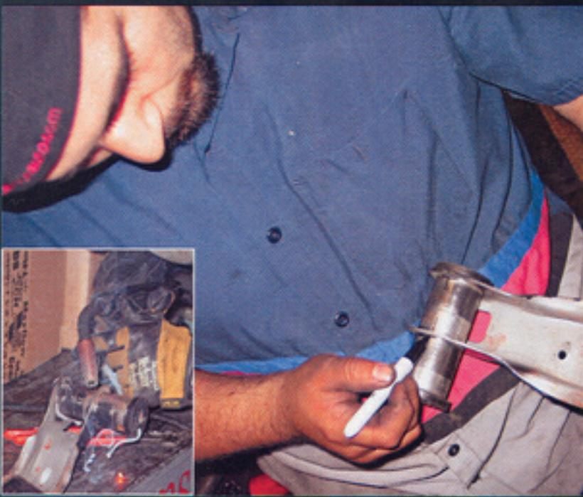
▲ The Surgeon operates on the crossmember's mounting tubes. Each tube is moved to its farthest-backward point, then Saul marks each place where the tube must be welded. After marking the tubes, he lays a bead of weld around the tube and secures it to the crossmember to ensure it won't move.
